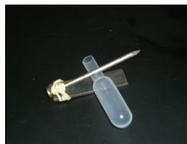
Figure 1. Bar and nail assembly- a nail is attached to a small bar of metal using a rubber band. Pliers will be used to seal the pipette bulb by squeezing the nail and metal bar together.
