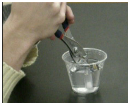
Figure 2. Pressure builds as the pipette bulb is sealed by squeezing the bar and nail assembly with pliers.
