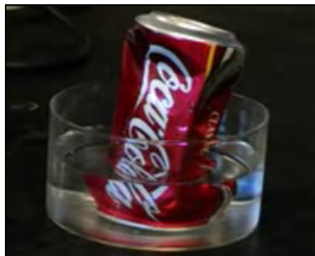
Figure 1. Can is crushed by atmospheric pressure.
